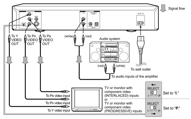
■ Switching the output signal (interlaced/ progressive) using the remote control (only when the SELECT (I/P) switch is set to "P")
